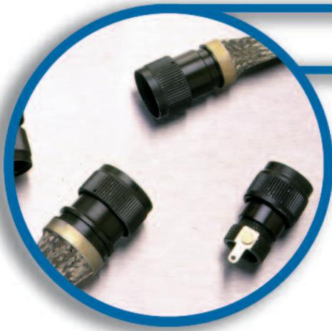
Connector Adaptors are designed for use with heat-shrinkable moulded shapes to provide high performance sealing, strain relief and EMC screening. A wide range of adaptor types are available to fit most designs of circular military connectors and are manufactured in a variety of materials and platings for optimum connector compatibility. They are particularly suitable for military, aerospace, marine and mass transit applications.
